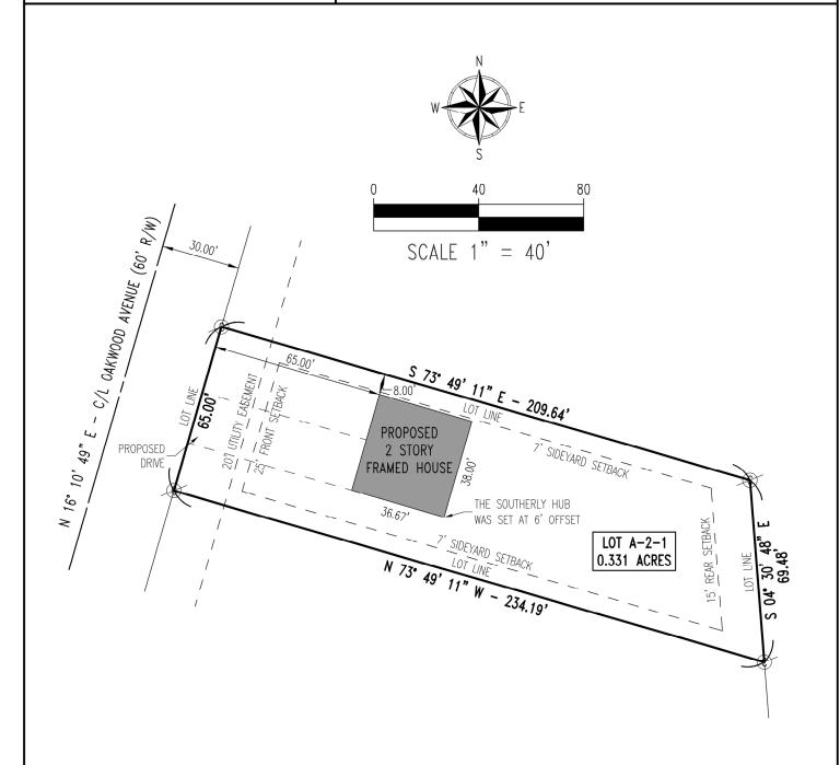
5' OFFSET WOOD HUBS WILL BE PLACED AT EACH CORNER OF OUTSIDE BOX OF PROPOSED HOUSE (UNLESS OTHERWISE STATED). THE DISTANCES SHOWN ARE FROM THE BUILDING TO THE LOT LINE. DISTANCES DO NOT GO TO THE EAVES OF THE HOUSE.
